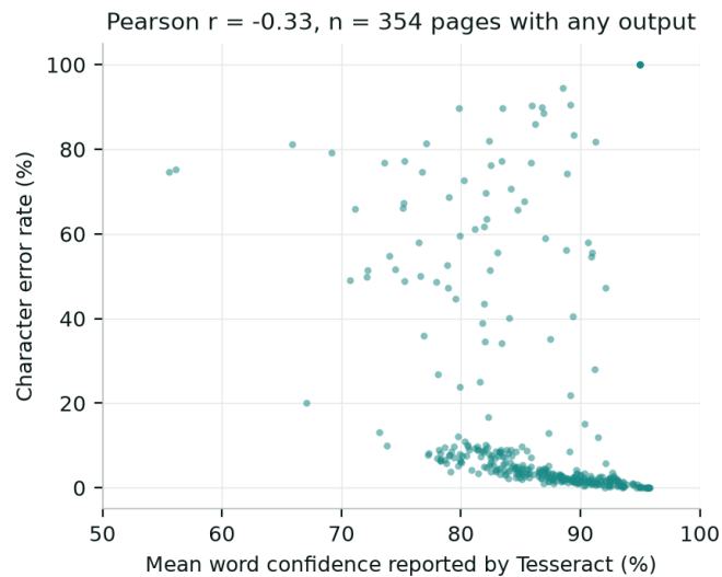
Figure 6: Mean word confidence provided by Tesseract against the measured character error rate, one point per page. Six pages for which Tesseract reported no confidence are omitted.
